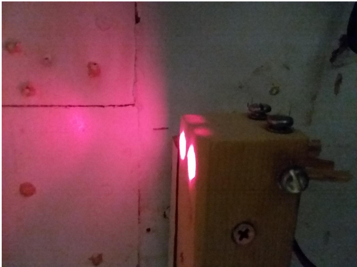
Figure 304 Laser mounting with adjustment screws
