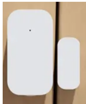
Figure 379 Door Open Sensor
