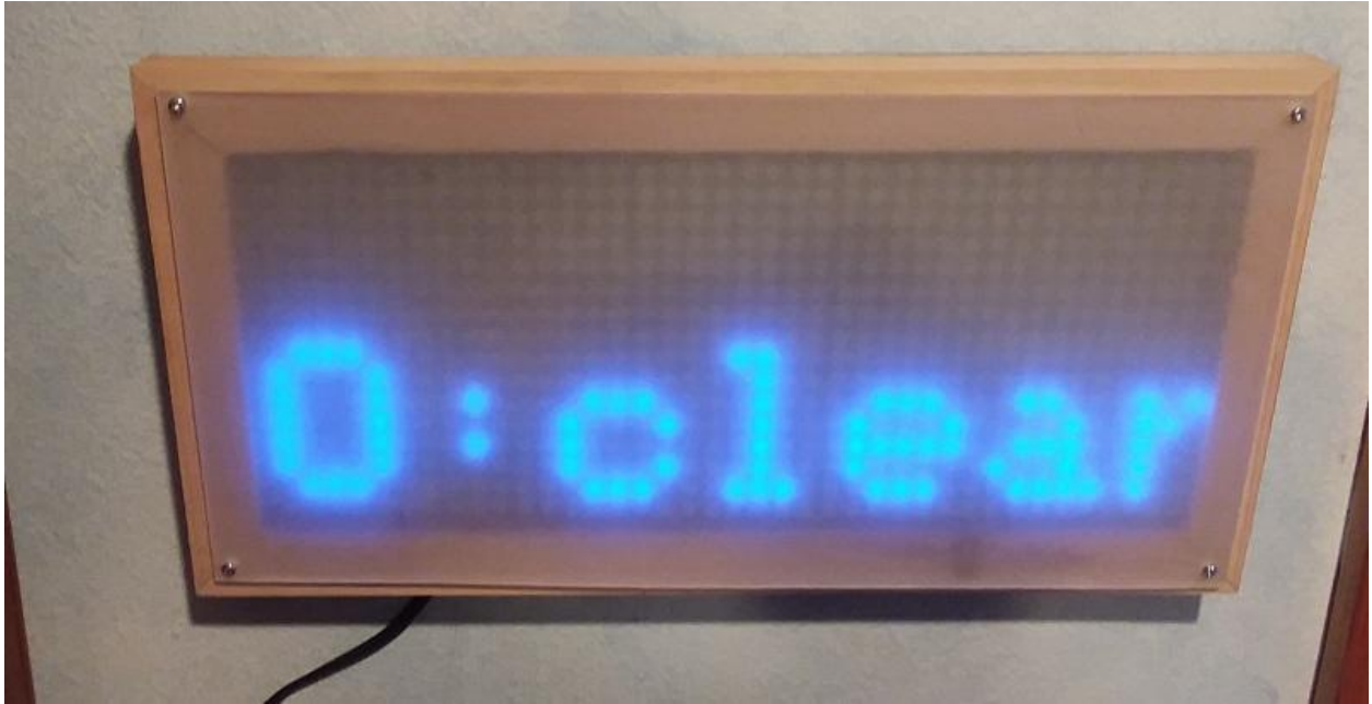
Figure 368 LED Sign with Diffuser Mounted
